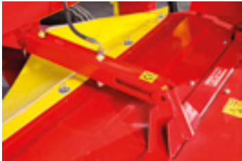
Hydraulic leveling piston.
